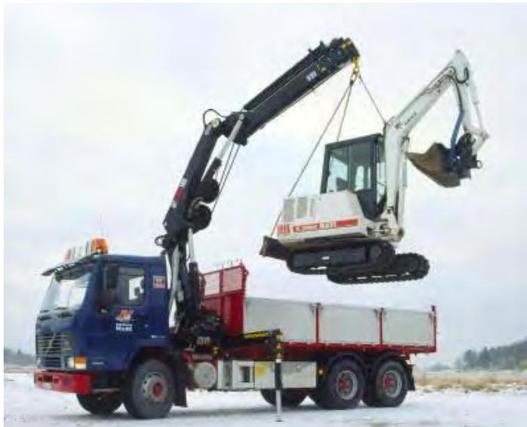
**Photo 3 - Lorry mounted Hiab and mini-excavator**
