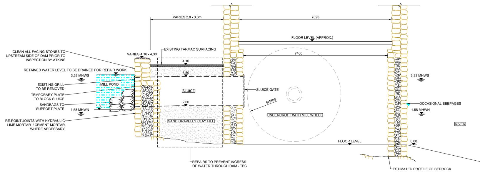
**X** TYPICAL DETAIL OF CAUSEWAY STRENGTHENING X-X
