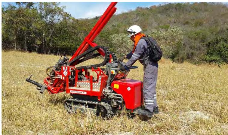
**Photo 5 - Tracked probing rig – (photo:Dando Drilling)**
